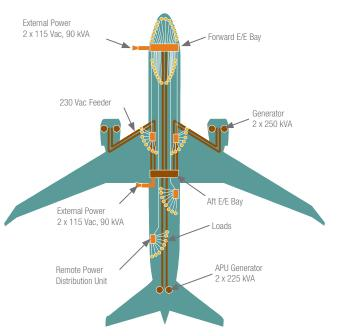
Remote Distribution: Solid-State Power Controllers and Contactors
