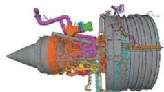
The ducting used to pass the pressurized air around the airplane employs check valves and pre-coolers, and is itself made of titanium, which adds hundreds of pounds of weight to the airplane.
