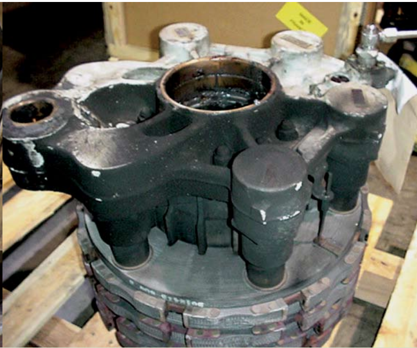
REMOVED BRAKE FOLLOWING FIRE FROM HYDRAULIC FLUID LEAK Figure 3
