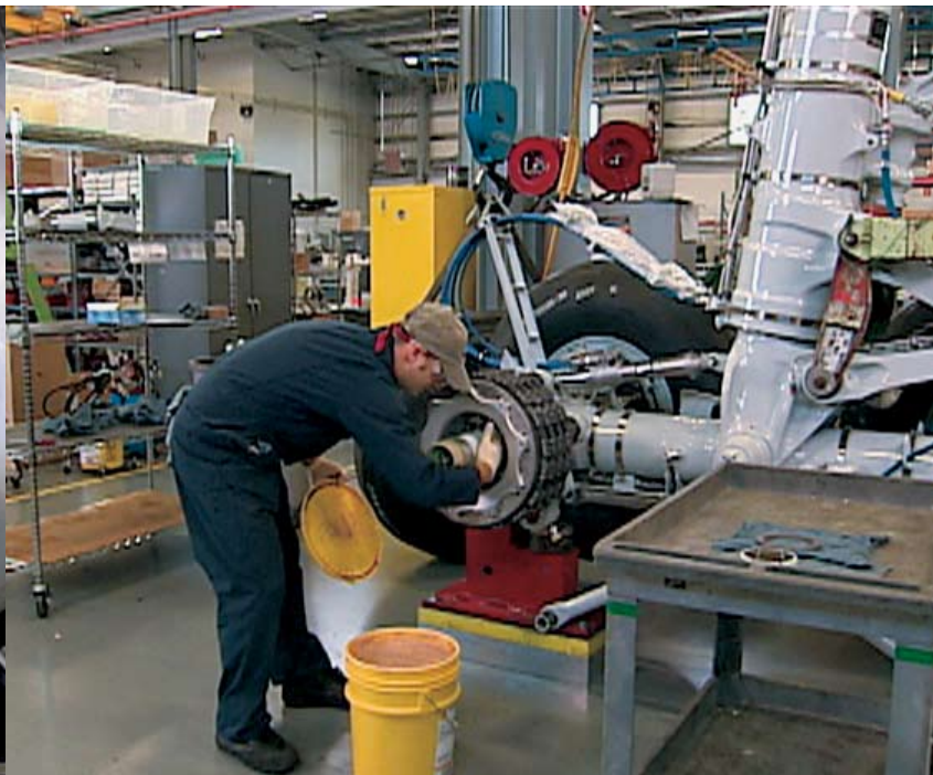
THIN LAYER OF GREASE BEING APPLIED TO BRAKE/AXLE SLEEVES Figure 5
