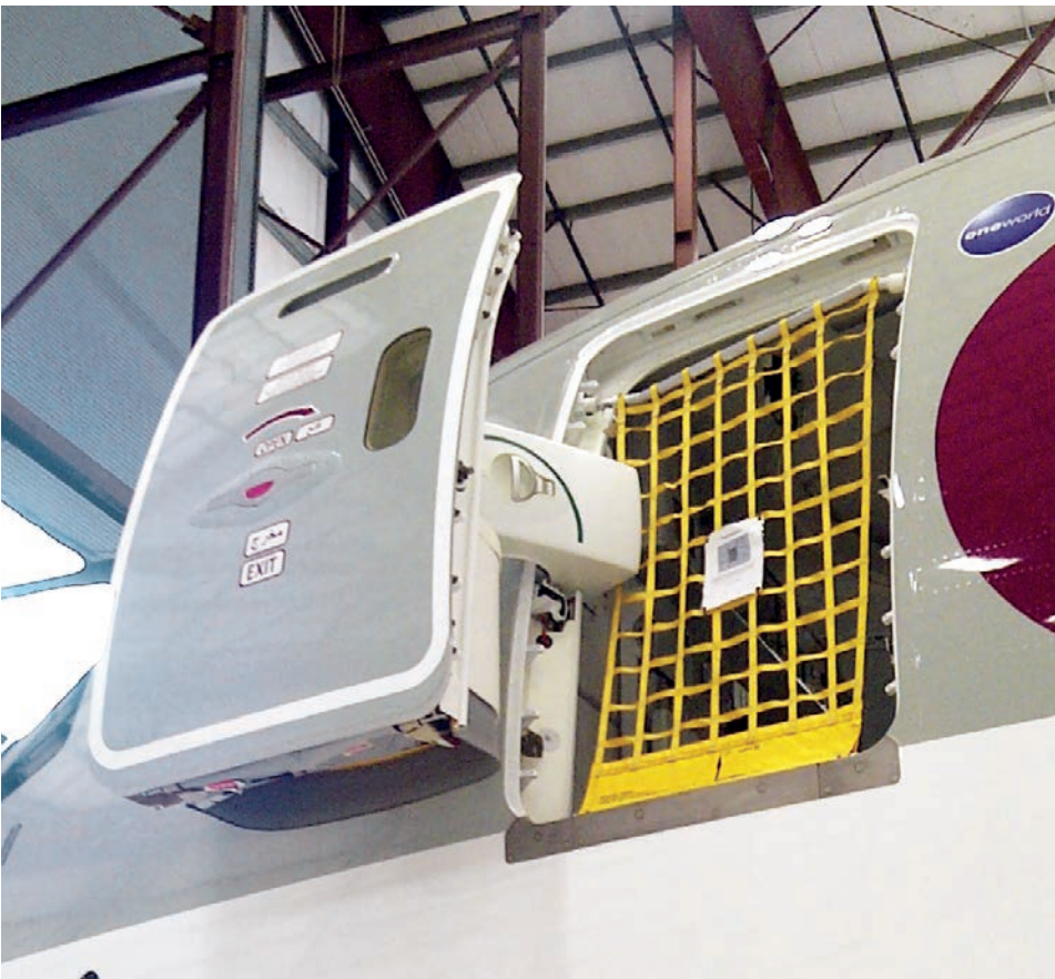
Figure 4: Personnel barrier for cabin entry door
