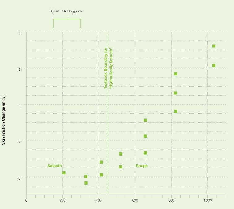
Equivalent sand-grain size, in microinches, on wing supersonic "rooftop."
