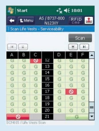
the RFID information wirelessly. This information then becomes an electronic record that travels with the airplane. RFID Integrated Solutions is the first fully integrated airborne automated identification technology program in commercial aviation.
