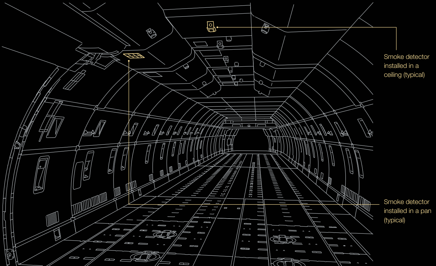
Figure 2: Class E main deck cargo compartment
