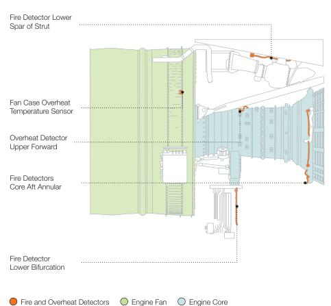
is designated as a zone, such as fire zone, flammable fluid leakage zone, or dry bay zone, according to the potential for the presence of flammable fluids and ignition sources (see fig. 1).
