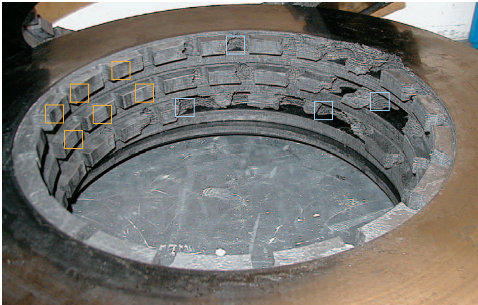
Figure 2: Damage to carbon brake disks caused by runway deicers
